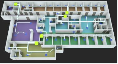
\*Template 1 with Gold Package details. Floor plan with ductwork and colored zoning added.
